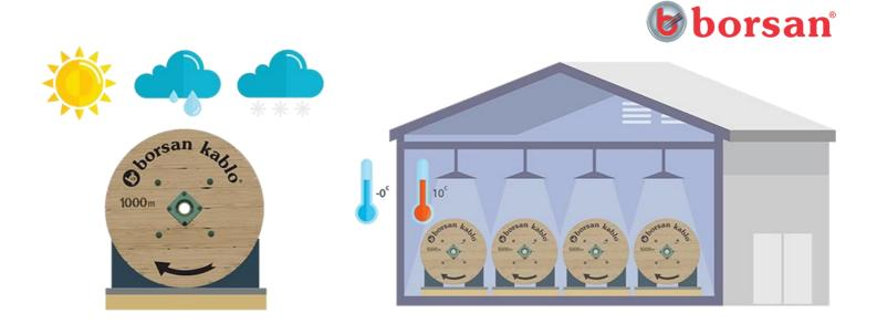
Normally, reel sizes are selected to nearly fill the gap between cables reeled around reels, flanges, and the most outside cable. In such a case, cable's weight helps maintain the reel's stability and position; but the cable's weight may cause flanges to get tilted in case reel is left motionless for a long time.
