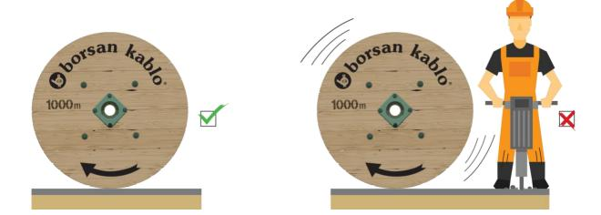
They should not be stored on rough, uneven, stony, indented areas. No storage must be allowed on soft surfaces (for instance, very sandy or wet earth).
