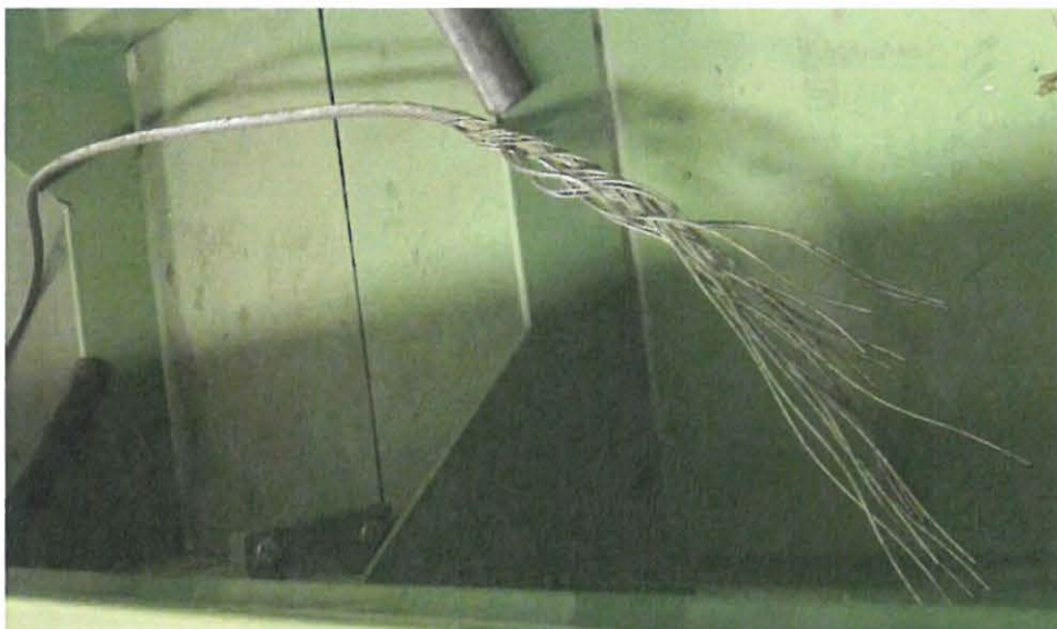
Photo 5 Broken conductor after tensile break test (anchoring clamps used)
