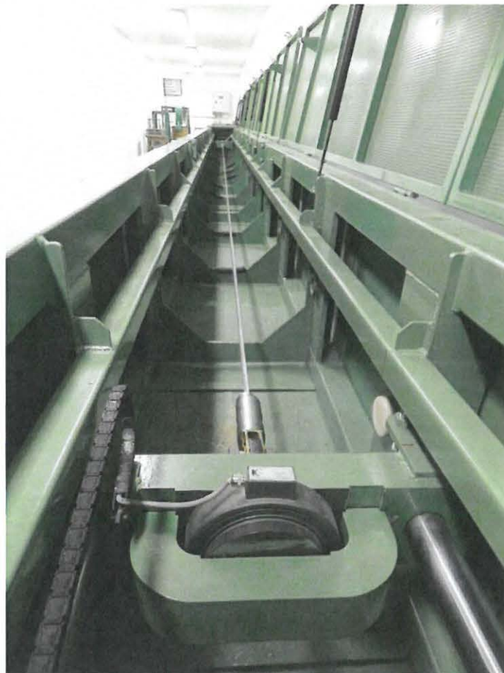
Photo 2 Test arrangement of the tensile break test with accessories
