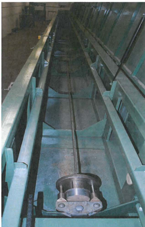
Photo 6 Test arrangement of the tensile break test with conical end fittings
