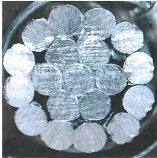
Photo 1 Cross-sectional view of the tested conductor
